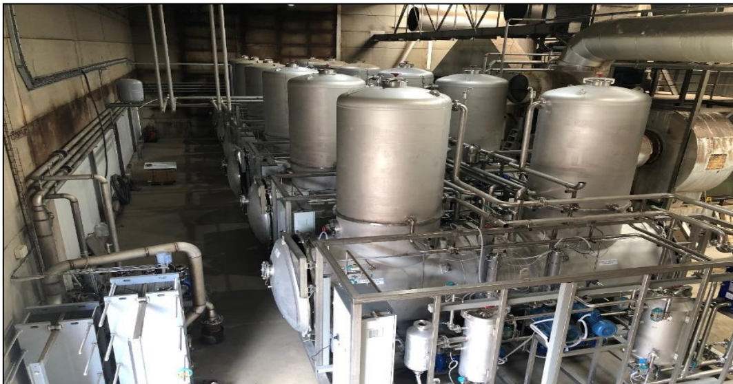
Figure 5. Evaporator with vertical distillation column
