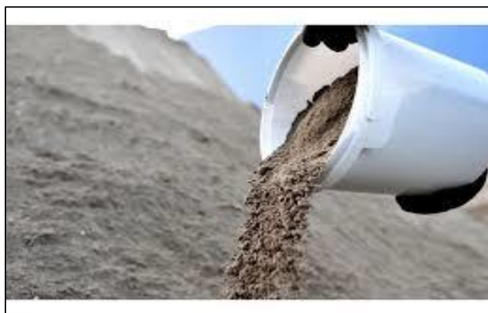
Figure 16. Hydrated poultry litter ash produced by BMC Moerdijk (Nutriman, 2020)
